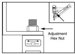
Figure 2. Single/bump fire adjustment.
